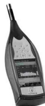
Fig. 3 Analyzer Type 2250
