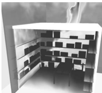
Fig. 6 Flame propagation outside the trade stand
