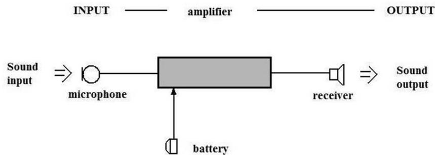
Fig. 2. Basic parts of hearing aid
