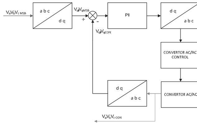
**Fig. 5 Block diagram of the PLL to synchronize national grid's converter with the ship's network**
