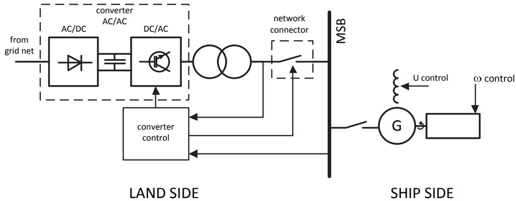
Fig. 3 STS system synchronization
