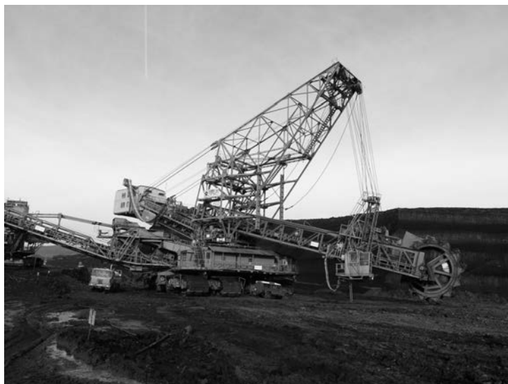
Fig. 1 Bucket-wheel excavator K800/N1/103
