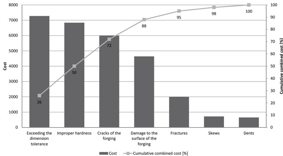
Fig. 1 The Pareto-Lorenz diagram of the cost of defects
