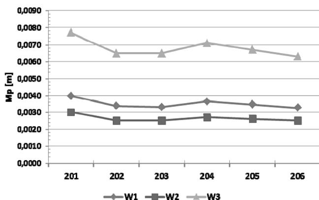
Fig. 3 Distributions of mean squared errors of points locations for the individual adjustment variants
