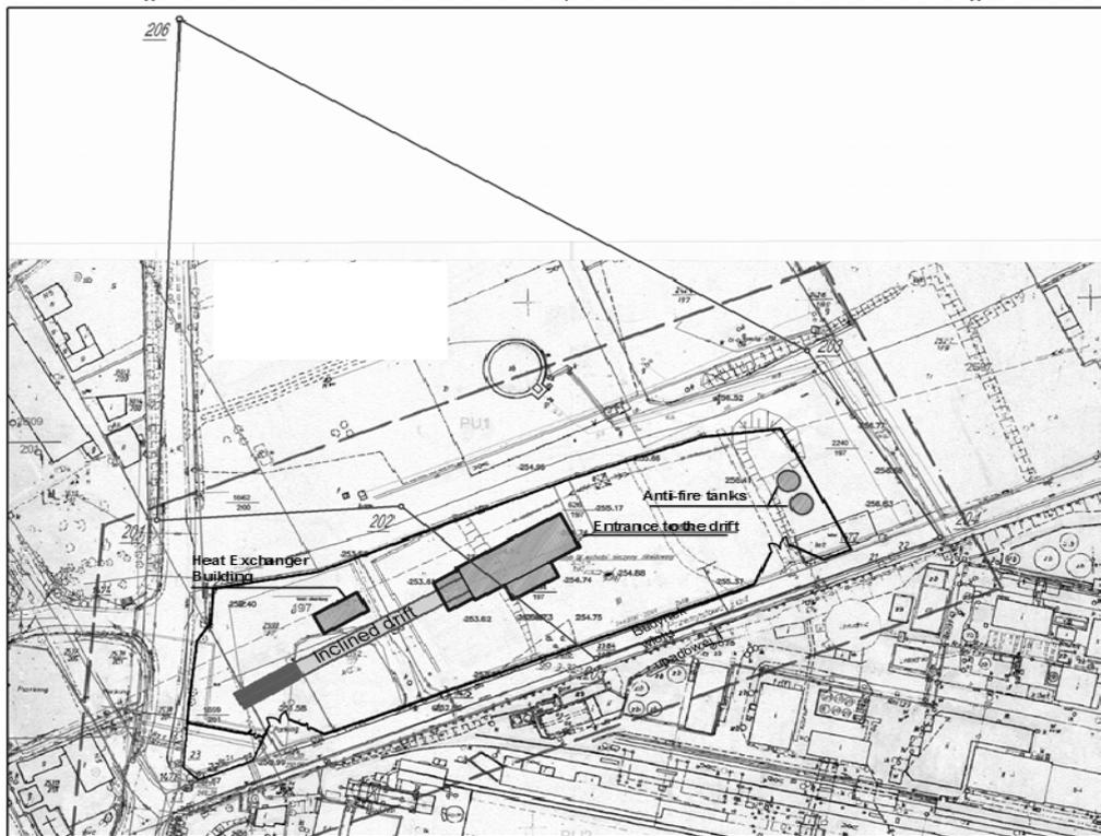
**Fig. 1** Arrangement of determined points of the realization control for the geodetic service of building of the inclined drift and associated objects
